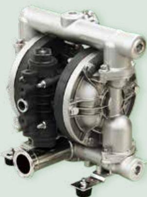
D250S □ F-X FDA Type Electro Polished HD SUS Pump. 1\frac{1}{2} " Sanitary Flange Connections. 190 L/min Max Flow Rate. (PTFE Diaphragms) 6.5mm Max Solids Size.
