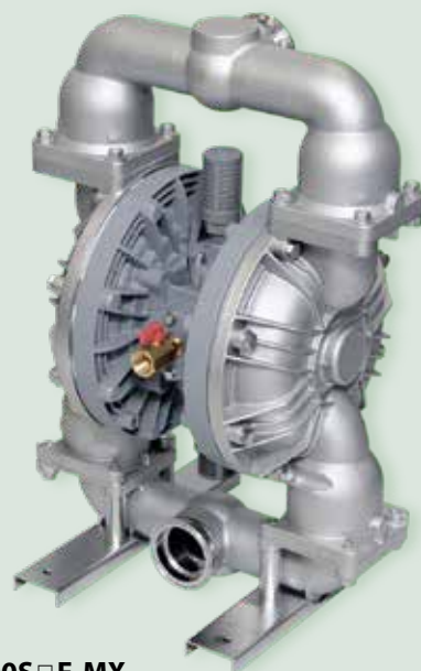
D500S □ F-MX FDA Type Electro Polished SUS Pump. 2\frac{1}{2} " Sanitary Flange Connections. 520 L/min Max Flow Rate. (PTFE Diaphragms) 8mm Max Solids Size.
